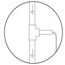
Additionally, make sure there is 9" clearance to allow removal of the electrode cell from the casing. Test by unscrewing the union if you are unsure you meet the clearance.
